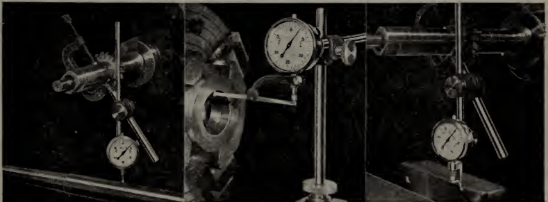
Showing simplicity of clamping indicator in place
